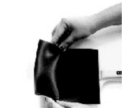
Attach the rubber. Begin with bottom edge and roll it onto the blade.
