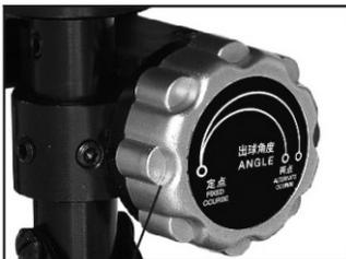
The angle of the serve can be adjusted by rotating the **Serve Angle Adjustment Knob**. Turn the knob counterclockwise for a smaller serve angle. Turn the knob clockwise to increase the angle.
