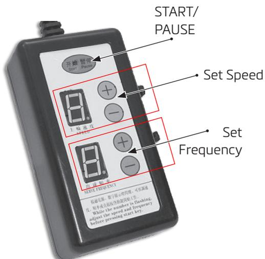
The Speed and Frequency of the balls can be adjusted by pressing the buttons on the Control Box.
